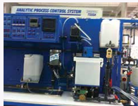
Teaching skids for pH monitoring and whole system put together by students after working on the individual module for chemical manufacturing.
